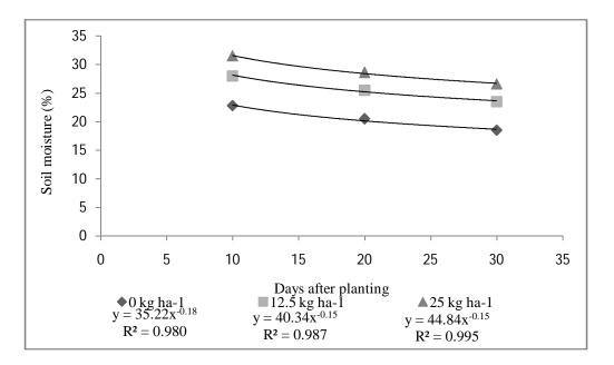
Figure 5: Effect of Three Hydrogel Doses in Soil Moisture Decrease at 30 of Depth
